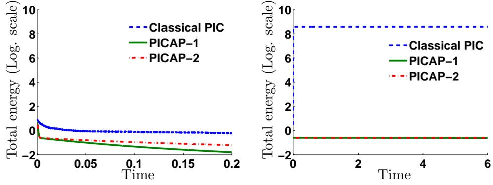
Figure 3: One-species periodic perturbation of a quasi-neutral Maxwellian plasma, with  $\lambda = 10^{-4}$ ,  $\omega = 10^4$ : total energy in log scale as a function of scaled time, with Classical PIC, PICAP-1 and PICAP-2 schemes. Left: resolved case:  $\Delta x = \lambda$  and  $\Delta t < \omega^{-1}$ ; right: under-resolved case:  $\Delta x = 10^{-2} > \lambda$  and  $\Delta t > \omega^{-1}$ .
