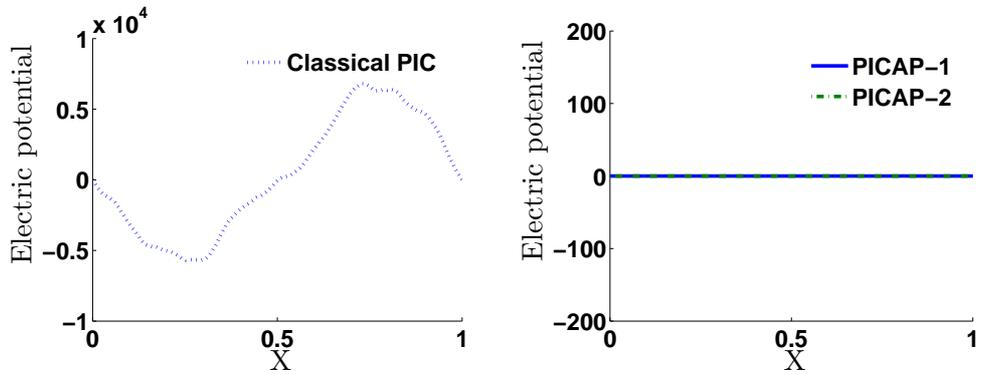
Figure 2: One-species periodic perturbation of a quasi-neutral Maxwellian plasma, under-resolved case:  $\Delta x = 10^{-2} > \lambda = 10^{-4}$  and  $\Delta t > \omega^{-1} = 10^{-4}$ . Electric potential as a function of position, with Classical PIC scheme (left), and PICAP-1, PICAP-2 schemes (right), at scaled time  $t = 0.2 = 2000\omega^{-1}$ .
