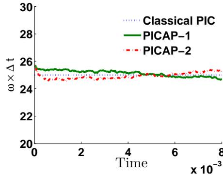
Figure 8: Two-species periodic perturbation of a quasi-neutral Maxwellian plasma, under-resolved case:  $\Delta x = 10^{-2} > \lambda$  and  $\Delta t > \omega^{-1}$ ,  $\varepsilon = 10^{-4}$ ,  $\lambda = 10^{-4}$ ,  $\omega = 10^6$ .  $\omega\Delta t$  as a function of scaled time, with Classical PIC, PICAP-1 and PICAP-2 schemes.
