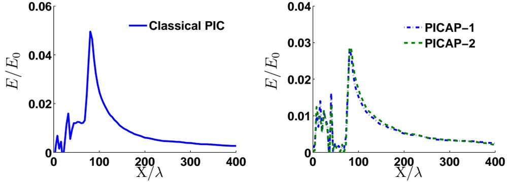
Figure 13: Plasma expansion test case. Simulation 2: space under-resolved and time resolved case:  $\Delta x = 4\lambda$  and  $\Delta t = 0.05\omega^{-1}$ . Electric field as a function of position, with Classical PIC scheme (left) and PICAP schemes (right), at time  $t = 30\omega_i^{-1}$ .
