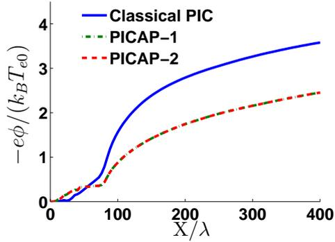
Figure 12: Plasma expansion test case. Simulation 2: space under-resolved and time resolved case:  $\Delta x = 4\lambda$  and  $\Delta t = 0.05\omega^{-1}$ . Electric potential as a function of position, with Classical PIC scheme and PICAP schemes, at time  $t = 30\omega_i^{-1}$ .
