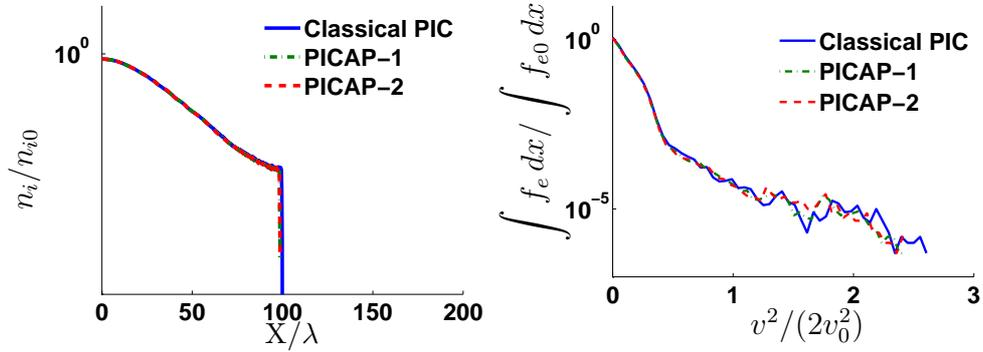
Figure 10: Plasma expansion test case. Simulation 1: resolved case (reference case):  $\Delta x = 0.2\lambda$  and  $\Delta t = 0.05\omega^{-1}$ . Ion density as a function of position in log scale (left) and electron velocity distribution as a function of  $v^2/(2v_0^2)$  (right) with Classical PIC, PICAP-1 and PICAP-2 schemes, at time  $t = 30\omega_i^{-1}$ . These pictures must be compared with Fig 10 (a) and Fig. 3 (a) (respectively) of reference [23].
