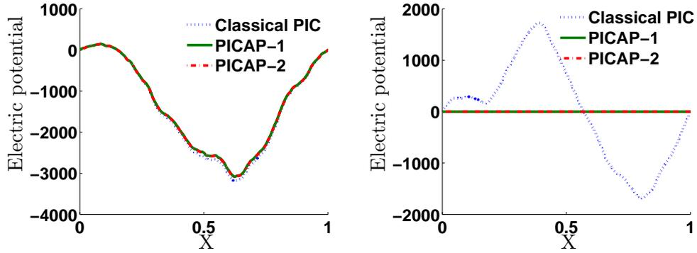
Figure 1: One-species periodic perturbation of a quasi-neutral Maxwellian plasma, resolved case:  $\Delta x = \lambda = 10^{-4}$  and  $\Delta t < \omega^{-1} = 10^{-4}$ . Electric potential as a function of position, with Classical PIC, PICAP-1 and PICAP-2 schemes. Left: at scaled time  $t = 10\omega^{-1} = 10^{-3}$  (all curves are identical) ; right: at scaled time  $t = 0.2 = 2000\omega^{-1}$ .
