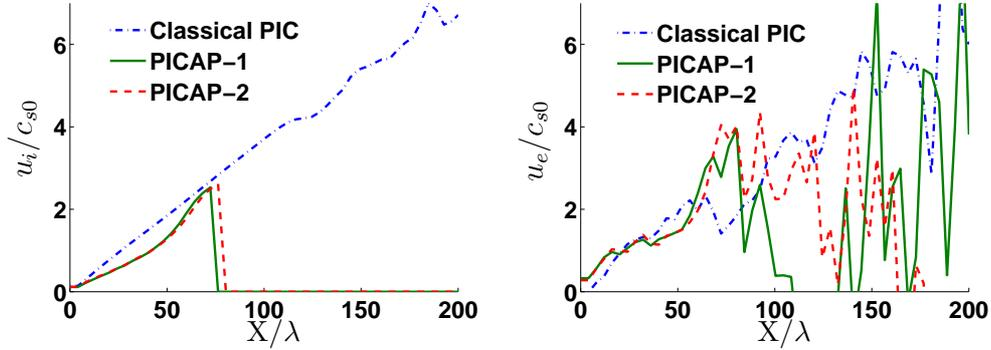
Figure 19: Plasma expansion test case. Simulation 3: space and time under-resolved case:  $\Delta x = 4\lambda$  and  $\Delta t = 3\omega_i^{-1}$ . Ion and Electron mean velocities as functions of position, with Classical PIC, PICAP-1 and PICAP-2 schemes, at time  $t = 30\omega_i^{-1}$  ( $c_{s0} = \sqrt{k_B T_{e0}/m_i}$ ).
