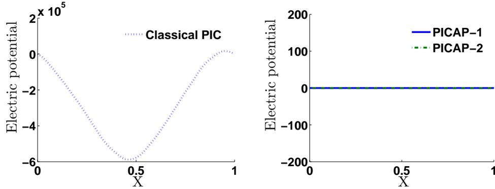
Figure 6: Two-species periodic perturbation of a quasi-neutral Maxwellian plasma, under-resolved case:  $\Delta x = 10^{-2} > \lambda$  and  $\Delta t > \omega^{-1}$  ( $\Delta t = 0.9\Delta x/v_{max} \approx 25\omega^{-1}$ ),  $\varepsilon = 10^{-4}$ ,  $\lambda = 10^{-4}$ ,  $\omega = 10^6$ . Electric potential as a function of position, with Classical PIC (left), PICAP-1 and PICAP-2 schemes (right), at scaled time  $t = 8 \times 10^{-3} = 8000\omega^{-1}$ .
