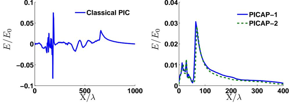
Figure 17: Plasma expansion test case. Simulation 3: space and time under-resolved case:  $\Delta x = 4\lambda$  and  $\Delta t = 3\omega^{-1}$ . Electric field as a function of position, with Classical PIC scheme (left) and PICAP schemes (right), at time  $t = 30\omega_i^{-1}$ .
