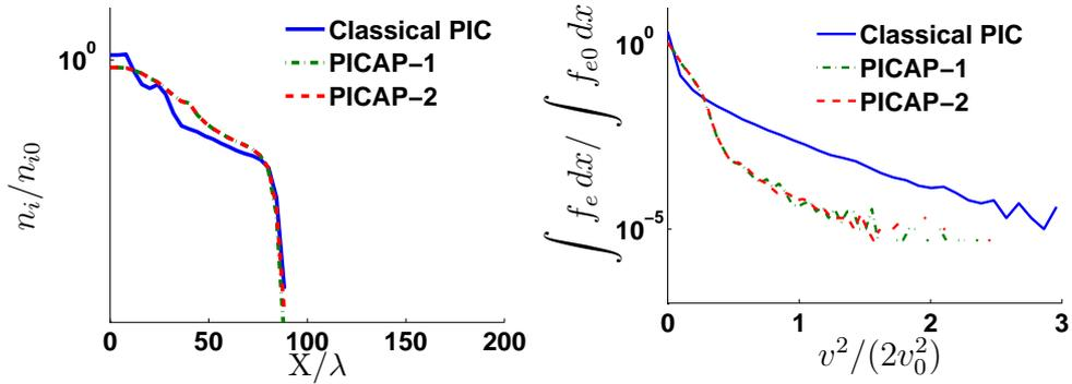
Figure 14: Plasma expansion test case. Simulation 2: space under-resolved and time resolved case:  $\Delta x = 4\lambda$  and  $\Delta t = 0.05\omega^{-1}$ . Ion density as a function of position in log scale (left) and electron velocity distribution as a function of  $v^2/(2v_0^2)$  (right) with Classical PIC and PICAP schemes, at time  $t = 30\omega_i^{-1}$ .
