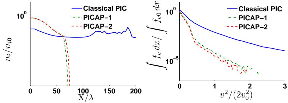
Figure 18: Plasma expansion test case. Simulation 3: space and time under-resolved case:  $\Delta x = 4\lambda$  and  $\Delta t = 3\omega^{-1}$ . Ion density as a function of position in log scale (left) and electron velocity distribution as a function of  $v^2/(2v_0^2)$  (right) with Classical PIC and PICAP schemes, at time  $t = 30\omega_i^{-1}$ .
