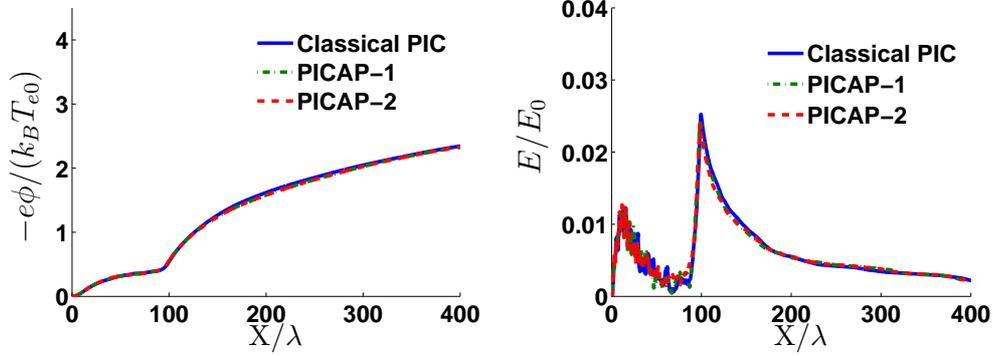
Figure 9: Plasma expansion test case. Simulation 1: resolved case (reference case):  $\Delta x = 0.2\lambda$  and  $\Delta t = 0.05\omega^{-1}$ . Electric potential (left) and electric field (right) as functions of position, with Classical PIC, PICAP-1 and PICAP-2 schemes, at time  $t = 30\omega_i^{-1}$ . These pictures must be compared with Fig 9 (a) and (b) of reference [23].
