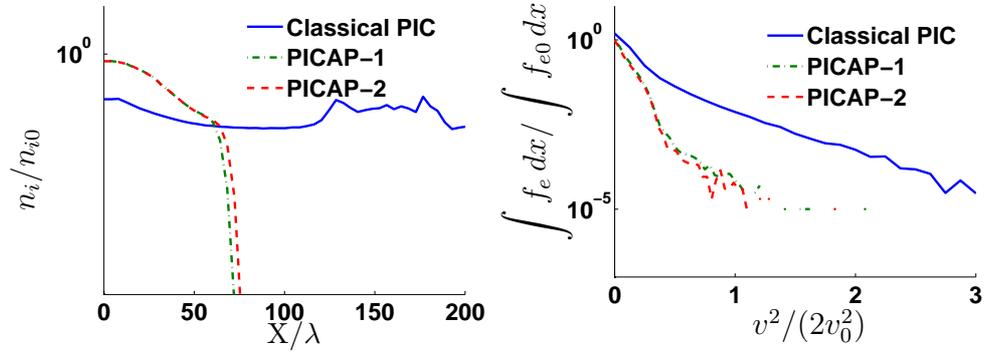
Figure 21: Plasma expansion test case. Simulation 4: space and time under-resolved case:  $\Delta x = 4\lambda$  and  $\Delta t = 3\omega^{-1}$  and small number of particles (1000 particles per mesh and per species). Ion density as a function of position in log scale (left) and electron velocity distribution as a function of  $v^2/(2v_0^2)$  (right) with Classical PIC and PICAP schemes, at time  $t = 30\omega_i^{-1}$ .
