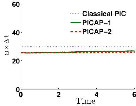
Figure 4: One-species periodic perturbation of a quasi-neutral Maxwellian plasma, under-resolved case:  $\Delta x = 10^{-2} > \lambda = 10^{-4}$  and  $\Delta t > \omega^{-1} = 10^{-4}$ .  $\omega \Delta t$  as a function of scaled time, with Classical PIC, PICAP-1 and PICAP-2 schemes.
