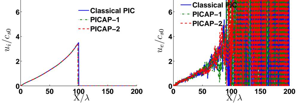
Figure 11: Plasma expansion test case. Simulation 1: resolved case (reference case):  $\Delta x = 0.2\lambda$  and  $\Delta t = 0.05\omega^{-1}$ . Ion and electron mean velocities as functions of position, with Classical PIC, PICAP-1 and PICAP-2 schemes, at time  $t = 30\omega_i^{-1}$  ( $c_{s0} = \sqrt{k_B T_{e0}/m_i}$ ). These pictures must be compared with Fig 10 (b) of reference [23].
