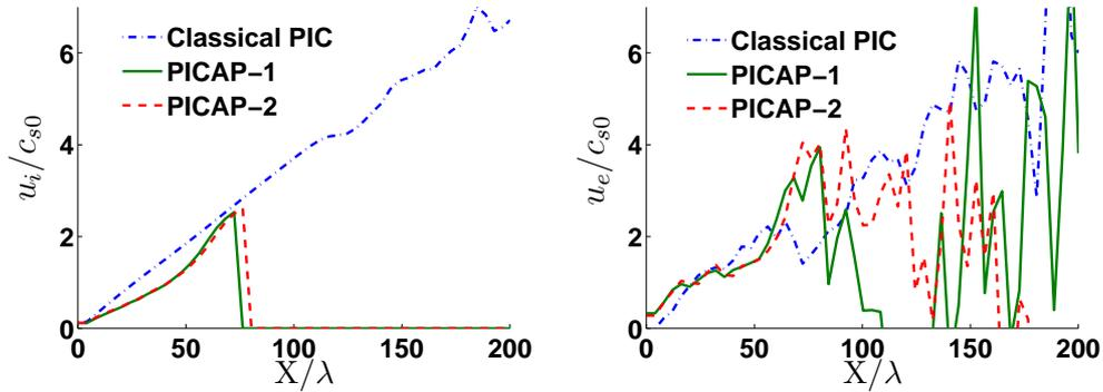
Figure 22: Plasma expansion test case. Simulation 4: space and time under-resolved case:  $\Delta x = 4\lambda$  and  $\Delta t = 3\omega^{-1}$  and small number of particles (1000 particles per mesh and per species). Ion and electron mean velocities as functions of position, with Classical PIC, PICAP-1 and PICAP-2 schemes, at time  $t = 30\omega_i^{-1}$  ( $c_{s0} = \sqrt{k_B T_{e0}/m_i}$ ).
